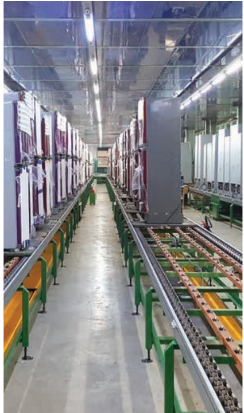
R600A REFRIGERATOR COMPRESSOR TESTING LINE AT WALTON. PHOTO CREDIT: ASHRAFUL AMBIA, EXECUTIVE DIRECTOR, WALTON
